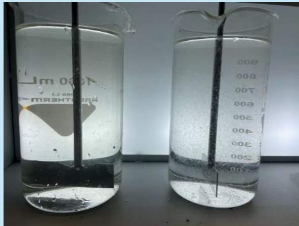
Figure 4: First minute of slow stirring comparison S AL (left) and CARB-CARB (right)
