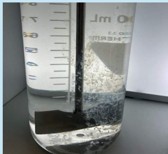
Figure 2: Loss of effectiveness of polysulphate in the absence of agitation
